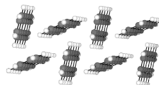
Figure 1. Solid-state order of unsubstituted pentacene.
