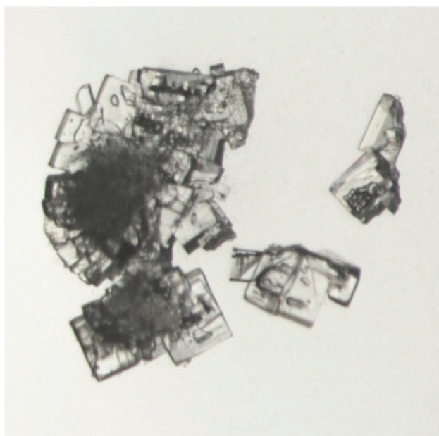
Fig. 1: 2EPNA crystals observed under the microscope. The large clump is about 1 mm \times 0.5 mm, and the individual single crystals are plates, about 0.1–0.2 mm across.
