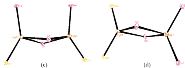
Figure 5. Two distinct structural motifs of \text{Hg}_2\text{I}_4\text{S}_4 type are observed in compound 2 . The \text{CH}_2\text{CH}_2\text{NH}_3\text{Cl} group attached to S is not shown.
