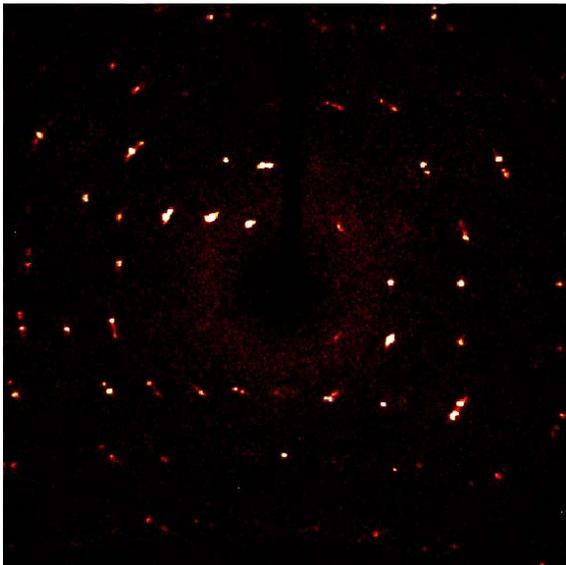
Figure 4.22 shows a  $2^\circ$  phi scan on a poor-quality crystal at  $+90$  in phi. The spot shape is poor, and the spots are very close together.
