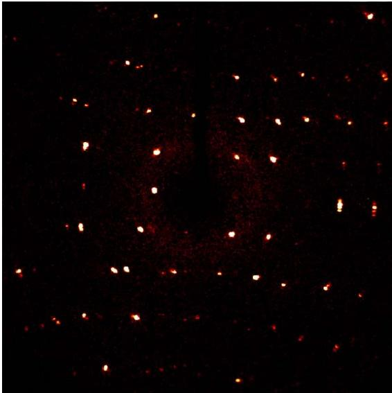
Figure 4.23 shows a  $360^\circ$  phi scan on a small crystal. The diffraction power of the crystal is poor, but with longer exposure times this is a reasonable candidate for data collection.
