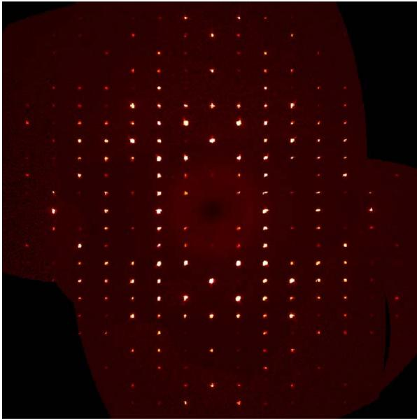
Figure 8.14 —A plane from a rotationally-twinned crystal, showing the two lattices
