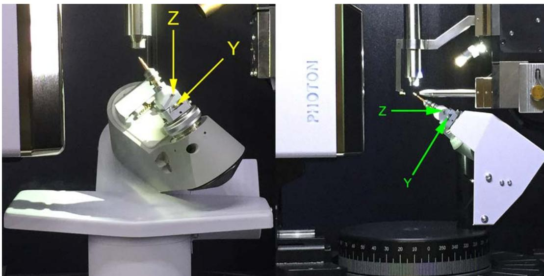
Figure 4.4 — Uncentered crystal as initially mounted
