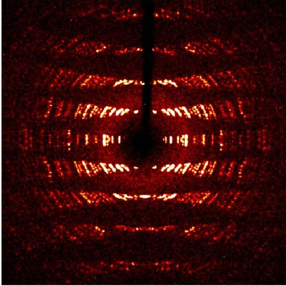
Figure 4.21 shows a 2° phi scan on a poor-quality crystal. The spot shape is poor, and some spots seem split.
