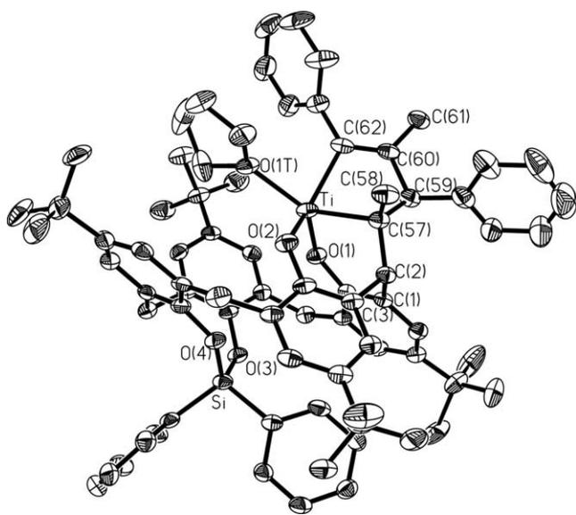
Fig. 5. An ORTEP diagram of the molecular structure of **16** showing 50% thermal ellipsoid probabilities.
