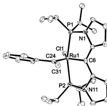
**Figure 2.** Thermal ellipsoid (50% probability) drawing of **10**.<sup>27</sup> All H atoms were omitted for clarity. Selected bond distances (Å) and angles (deg): Ru1–C6, 1.911(4); Ru1–C24, 2.052(4); Ru1–P1, 2.3191(11); Ru1–P2, 2.3355(11); Ru1–Cl1, 2.4288(11); C6–Ru1–C24, 87.45(16); C6–Ru1–P1, 84.22(13); C24–Ru1–P1, 93.25(11); C6–Ru1–P2, 83.97(13); C24–Ru1–P2, 93.15(11); P1–Ru1–P2, 166.29(4); C6–Ru1–Cl1, 130.50(12); C24–Ru1–Cl1, 142.03(12); P1–Ru1–Cl1, 90.19(4); P2–Ru1–Cl1, 92.20(4).
