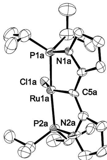
**Figure 1.** Thermal ellipsoid (50% probability) drawing of **2** (only one molecule is shown here).<sup>27</sup> All H atoms were omitted for clarity. Selected bond distances (Å) and angles (deg) for one of the three nonequivalent molecules: Ru1A–C5A, 1.918(10); Ru1A–P1A, 2.282(2); Ru1A–P2A, 2.300(2); Ru1A–Cl1A, 2.416(2); C5A–Ru1A–P1A, 84.3(3); C5A–Ru1A–P2A, 84.7(3); P1A–Ru1A–P2A, 168.33(10); C5A–Ru1A–Cl1A, 146.6(2); P1A–Ru1A–Cl1A, 93.78(10); P2A–Ru1A–Cl1A, 97.59(9).
